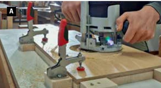
**A Vertical toggle with open arm and horizontal base plate**
