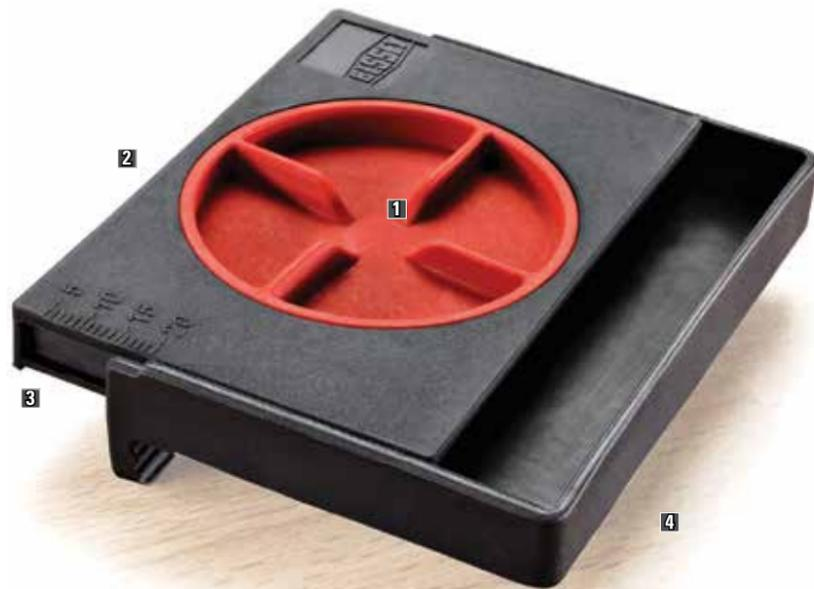
For fast and simple setup of flooring installations. Simply turn the dial to set the desired gap on your spacers and insert between wall and flooring. When the job is done a simple twist of the dial constricts the spacer for easy removal.
