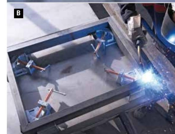
Check out WSM Welders' angle clamps in action!
