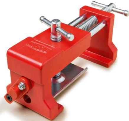
The cabinetry clamp is designed to combine the multiple steps of face frame cabinet installation into one easy process. It works on stiles 1-1/2 to 2 IN. and up to 1-1/4 IN thick (each). Face frame stiles can be tightened, aligned, pre-drilled and fastened while the clamp is held in place. The clamp holds the individual cabinet edges together while also keeping the faces along the joint flush.
